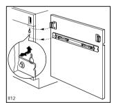
Mount the decor panel by inserting the two pivots of the cross-bar into the slotted holes of the door.
